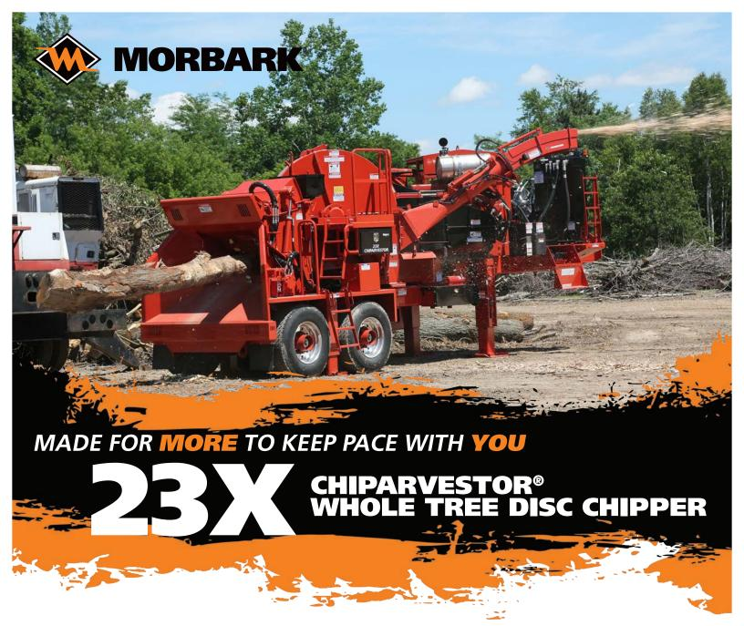
Morbark 23X Chiparvestor® whole tree chippers are built to last. The improved chipper hood design allows for better access to the disc during inspections and maintenance, while the 23" (58.42 cm) chipping diameter tackles some of the larger trees. Like the previous Model 23 Chiparvestors, the 23X uses a 75" (190.5 cm) diameter x 5" (12.7 cm) thick chipper disc to chip large volumes of wood, while the built-in dirt separator with deflector keeps the end product clean.
